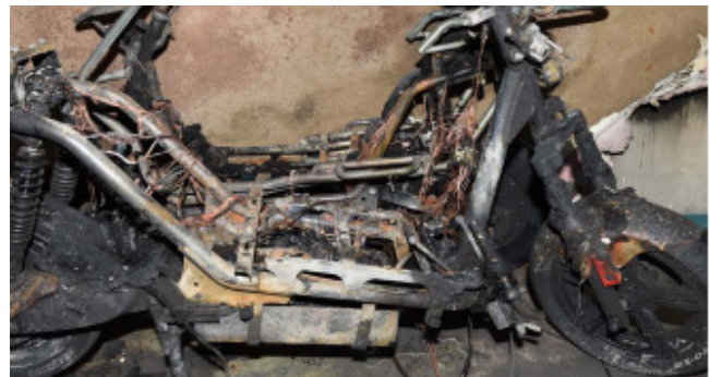
Fire involving lithium-ion battery powered eBike
