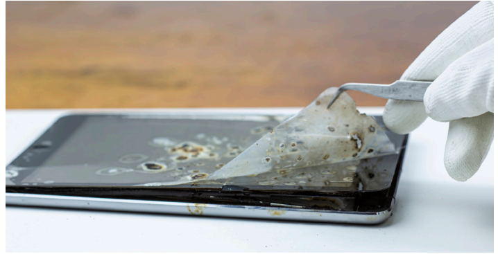
Evidence of overheated Lithium-ion phone battery.
